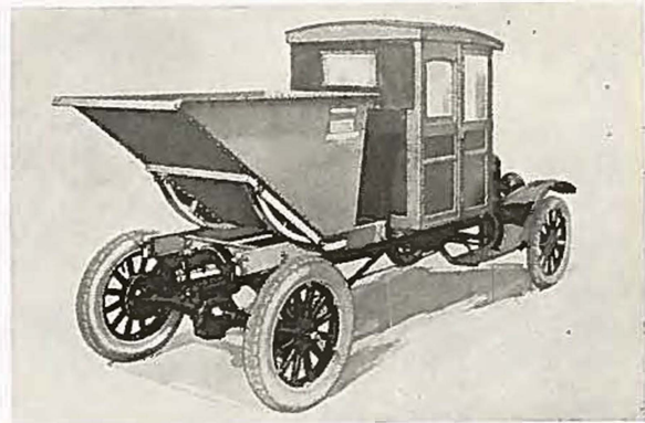
Automatic Hopper Type Body BUILT IN 1 1-2 TO 2 YARD CAPACITY--SINGLE OR DUAL TYPES
